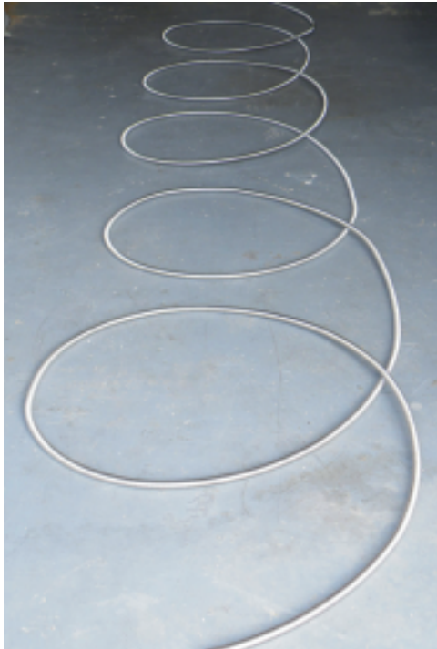
Coiled flexible stainless steel tube which could be used to form a heat exchanger on the bed of the brook.
