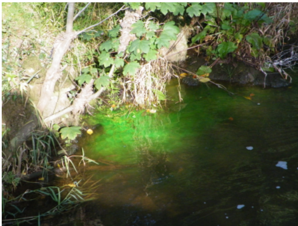
Below, the dye emerging in the river east of the bridge, though the exact point of entry is not easy to see.
