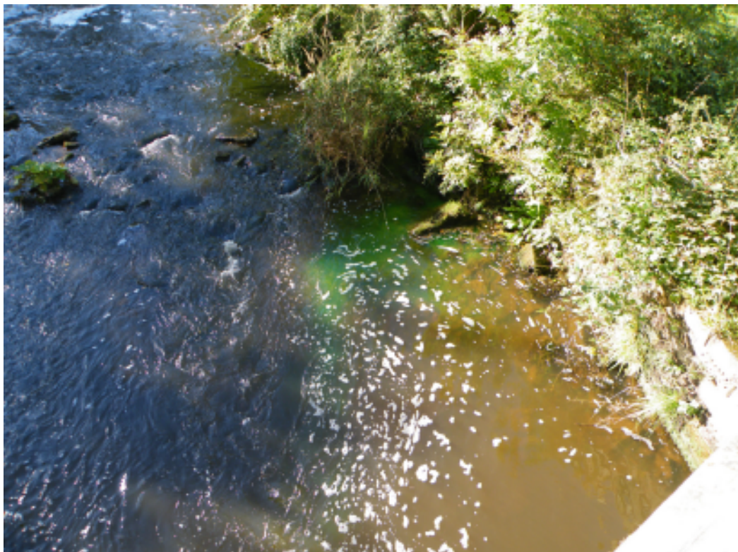
Below, the dye emerging in the river west of the bridge, though again, the exact point of entry is not easy to see.
