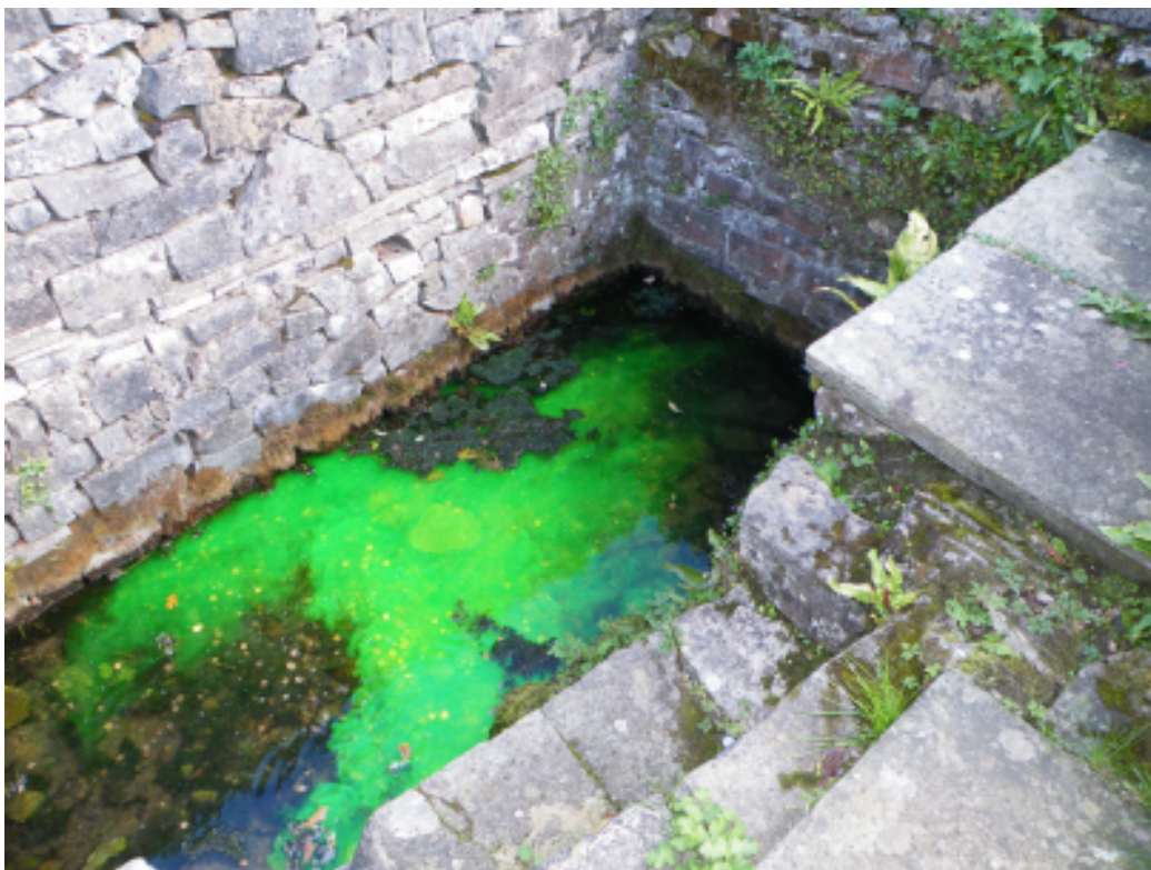
Above, viewed from the north west, drain dye entering Wishing Well from the west, and flowing to the south while the north end remains clear.
