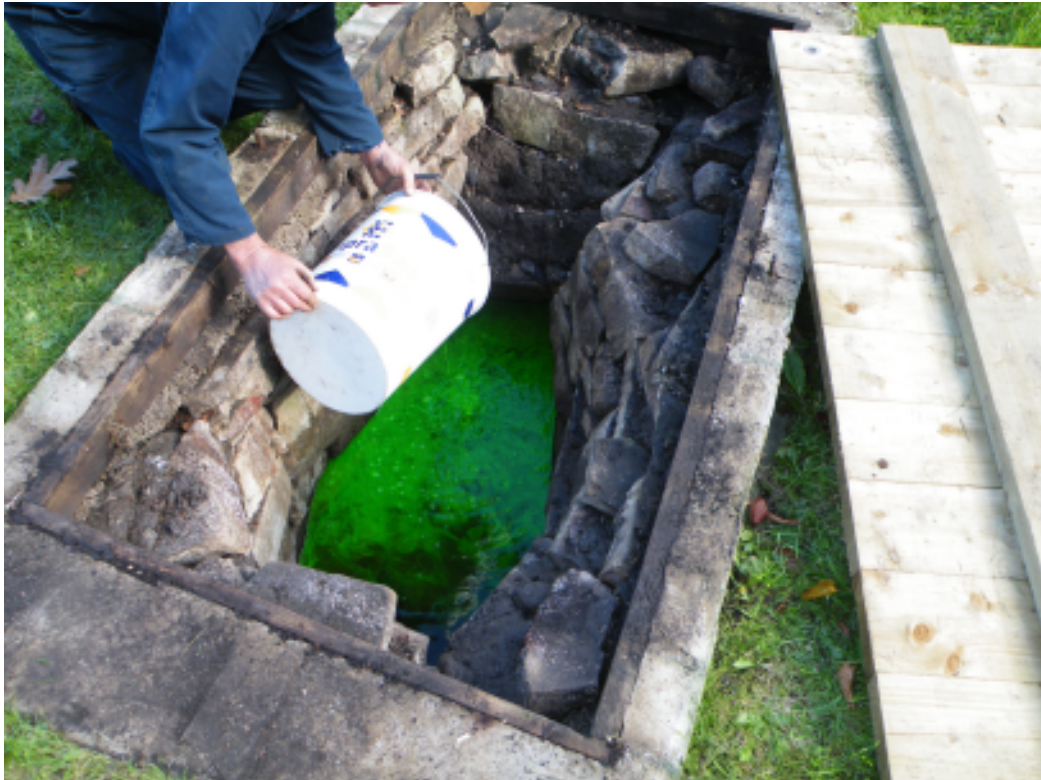
Above, viewed from the east, drain dye poured into Coffin Well to see if this has a direct link to the river.
