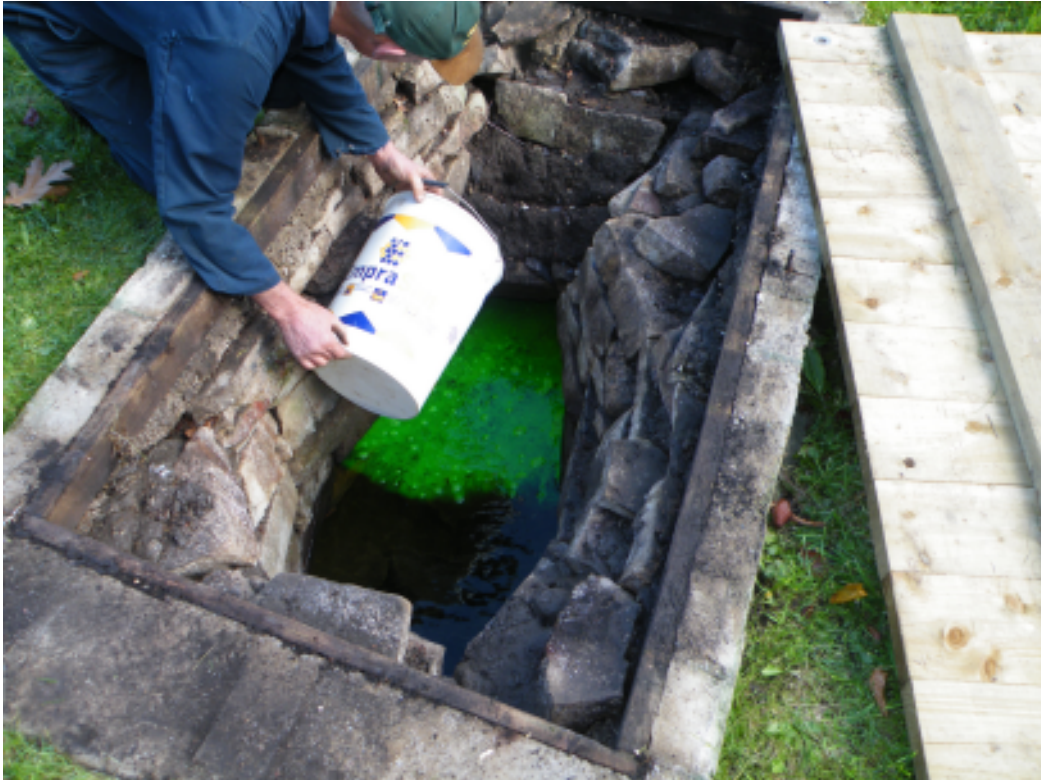
Above, drain dye poured into the east end of Coffin Well.
