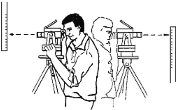
Figure 4.1 Using a dumpy or surveyor's level and staff to measure head (courtesy of BHA)
