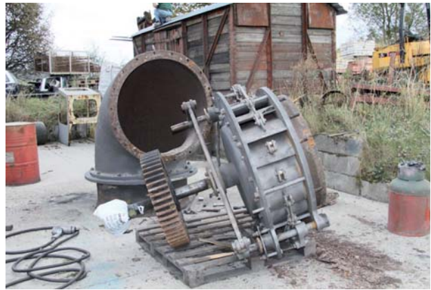
Figure 5.2 The Frances turbine from Flewitt's Mill awaiting refurbishment in winter 2009 (photo courtesy of R. Griffiths)
