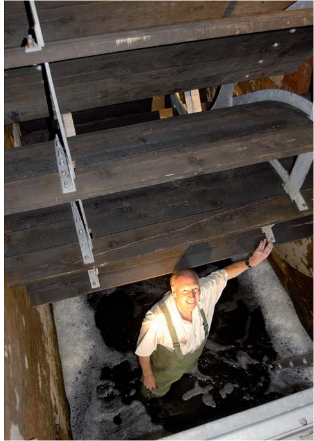
Figure 5.4 A modern waterwheel manufactured by Hydrowatt of Germany recently installed at Lemsford Mill, Hertfordshire (photo courtesy of Ramblers Worldwide Holidays)
