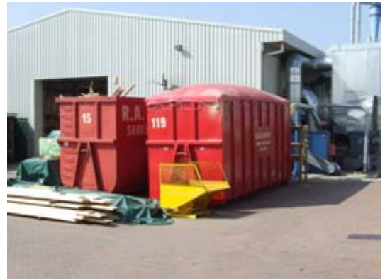
Right, Central Joinery's wood recycling – on the right hand-side, the wood incinerator used to heat the shop floor; in the foreground, 2 skips to collect block wood waste (skip on the left) and wood dust (skip on the right)
